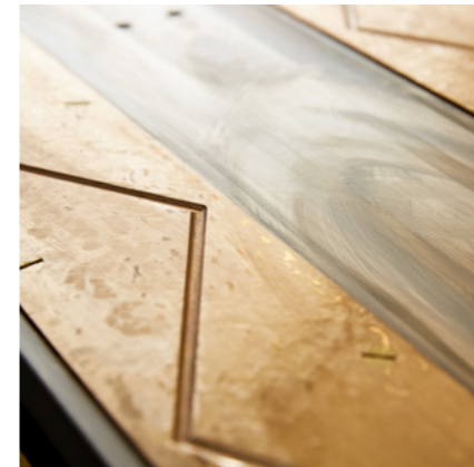
Among others, expensive bronze guideways – scraped by hand – warrant the longevity of our machines
